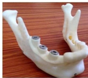
Dental drill guide fabricated on rapid prototyping machine (EDEN 260V) & fitted with SS 316L sleeve
